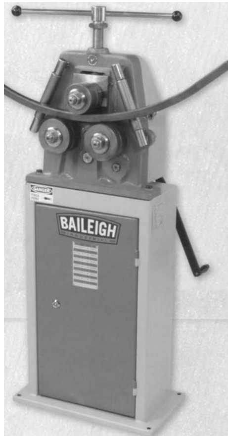
Fig. 4 Manually powered three-roll bender. Courtesy of Baileigh Industrial Inc.
