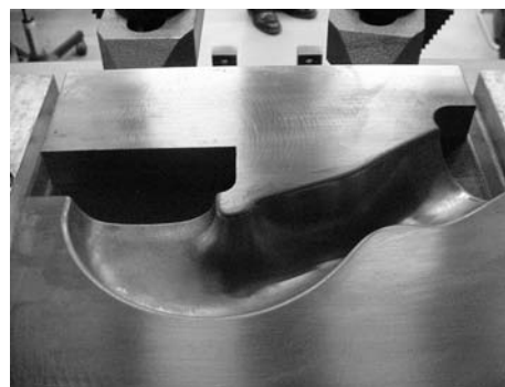
Fig. 1 Low-volume tooling produced by the rapid manufacturing method metal copy. Courtesy of Prototol AB, Sweden
