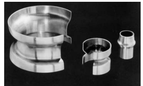
Fig. 6 Thermally formed components showing change in diameter and wall thickness (Ref 8)
