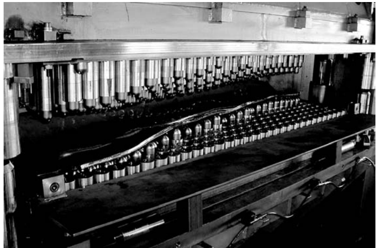
Fig. 3 Flexible multipoint forming in which the die pins replace both die and stamp. (a) Different modes of multipoint forming can be either passive or produces an active pressure toward the stamp. (b) Flexible multipoint forming of 16 mm (0.63 in.) stainless steel sheet. Courtesy of Unformtechnik Stade GmbH, Germany
