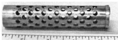
Fig. 8 Example of a 4130 cylinder given multiple perforations in a single explosive operation. Source: Ref 17
