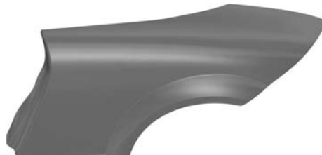
Fig. 35 Part geometry (computer-aided design surfaces) of a rear fender
