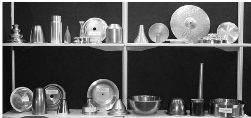
Fig. 1 Various components produced by metal spinning. Courtesy of Leifeld USA Metal Spinning, Inc.
