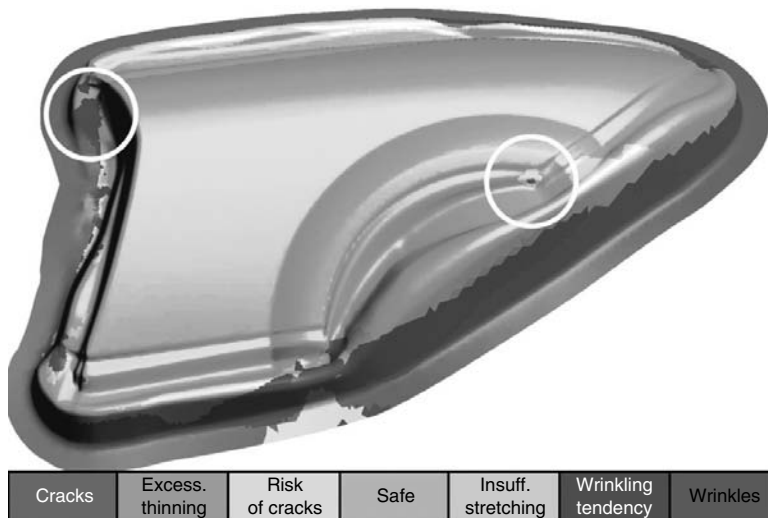
Fig. 41 Result of a one-step simulation. The circled area on the left shows a risk of wrinkles on the addendum, very near to the part boundary. The circled area on the right shows a crack.
