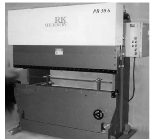
Fig. 8 Hydraulic press brake with 1.8 m (6 ft) bed length and 440 kN (50 tonf) load capacity with a 4 kW (5 hp) motor
