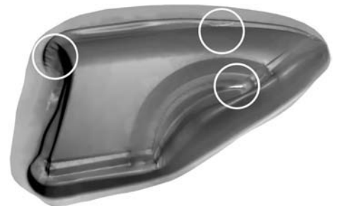
Fig. 42 Result of an accurate incremental try-out simulation of the complete stamping process. Thinning zones shown by two circled areas on the right. Wrinkling is indicated by the circled area on the left.
