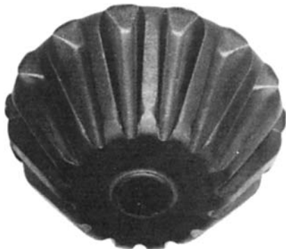
Fig. 47 Warm precision forging of a 1.25% C ultrahigh-carbon steel billet into a bevel gear. Forging temperature was 650\ ^\circ\text{C} ( 1200\ ^\circ\text{F} ).
