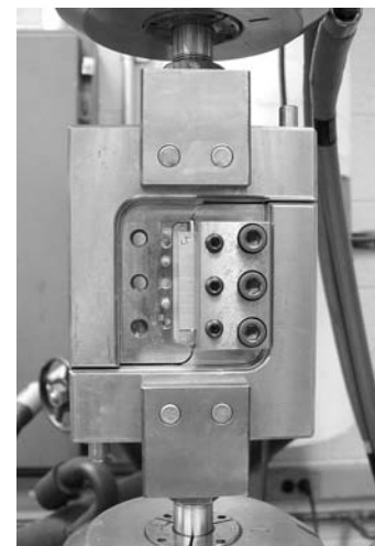
Fig. 4 Simple shear test device
