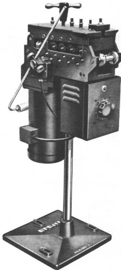
Fig. 9 Powered pedestal-type stock straightener
