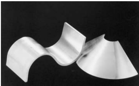
Fig. 7 Three-dimensional thermally formed components (Ref 8)
