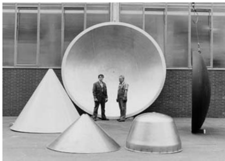
Fig. 10 Photograph of very large-diameter (~2 m, or 6.5 ft) cone- and dish-shaped components produced by the Leifeld Company. Courtesy of Leifeld USA Metal Spinning, Inc.
