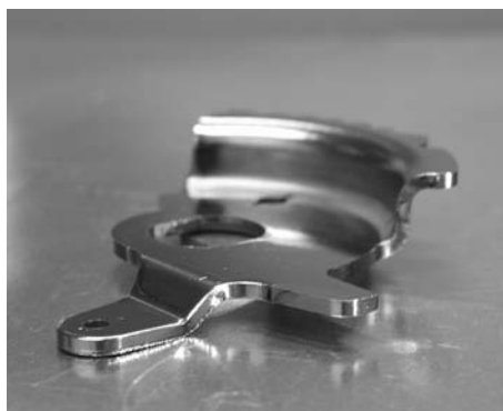
Fig. 14 A sample two-dimensional part made by fine-blanking
