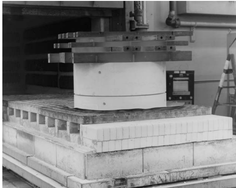
Fig. 7 Creep forming a part for the B-737 in a ceramic die using a conventional furnace. The titanium is pushed into the correct shape through the application of heat, weight, and time.
