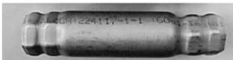
Fig. 6 Example of a 6061-T6 32 mm (1.25 in.) diameter, 1 mm (0.04 in.) wall thickness tube electromagnetically crimped onto four nuts using four electromagnetic discharges and a coil similar to that shown in Fig. 5(a). The nuts are tight after forming and after destructive testing.
