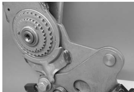
Fig. 28 Fine-blanked central gears of car seat adjuster
