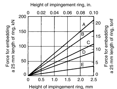
Fig. 26 Force required for embedding impingement rings of various heights into several different work metals. A, stainless steel; B, prehardened alloy steel, C, mild steel, half-hard brass, hard copper, 6xxx aluminum alloys in the H temper; D, soft copper; series 6000 aluminum alloys, half hard; E, commercially pure aluminum, H temper
