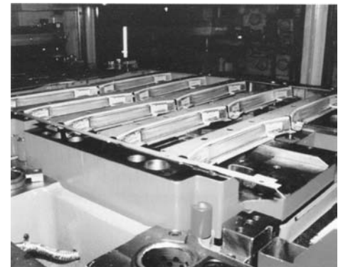
Fig. 3 Tandem part production on progressive die machine. Courtesy of Müller Weingarten
