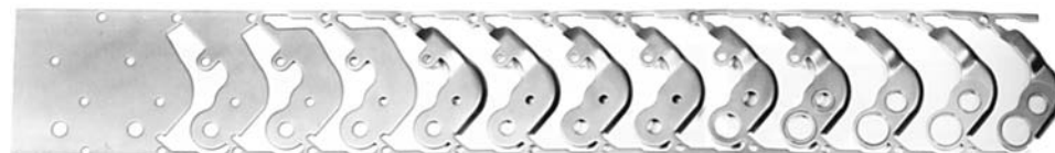
Fig. 2 Combined sequential production of a structural part with progressive die technology
