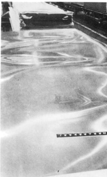
Fig. 3 Center buckles in a random pattern. Source: Ref 1
