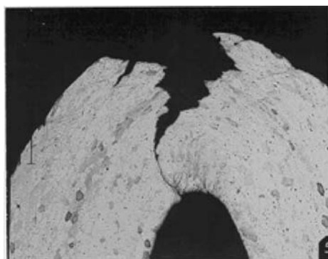
Fig. 1 Example of an aluminum alloy fractured in a flat-hemming operation. Source: Ref 3
