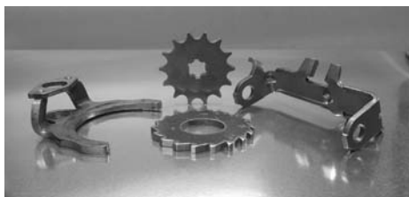
Fig. 1 Fine-blanked parts (a) assembled as the main components of an automatic car window. (b) Other fine-blanked parts
