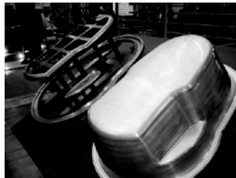
Fig. 13 Bathtub measuring ~1500×1000 mm (60×40 in.) and the corresponding support tool
