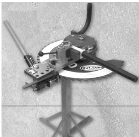
Fig. 3 Manual rotary draw tube bender. Courtesy of Baileigh Industrial Inc.
