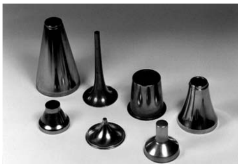
Fig. 4 Photograph of conical components that were produced by metal spinning. Courtesy of Leifeld USA Metal Spinning, Inc.
