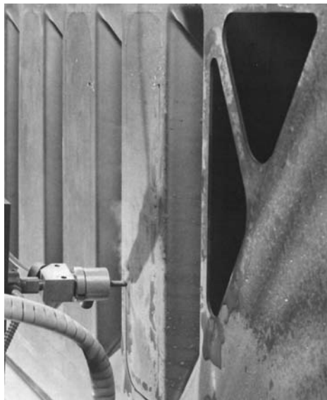
Fig. 17 Profiling of titanium for aerospace applications using an abrasive waterjet. Courtesy of Flow Systems, Inc.
