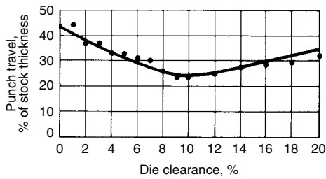
Fig. 27 Distance of punch travel through 3.2 mm (1/8 in.) thick flat aluminum stock (hardness, 73 HRB) for complete severance
