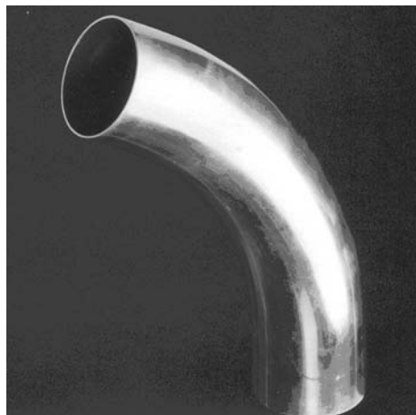
Fig. 13 Tube bend manufactured by laser forming (Ref 8)
