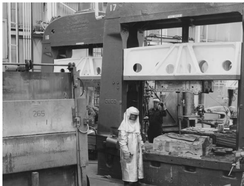
Fig. 20 Drop hammer forming showing oven next to the drop hammer
