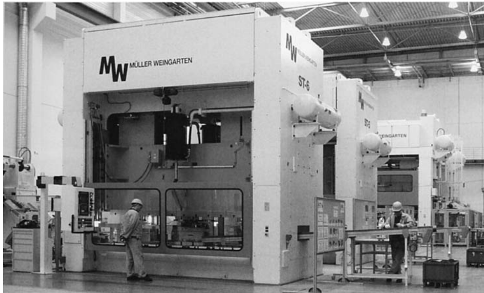
Fig. 9 Classic in-line arrangement of automatic blanking and forming machine
